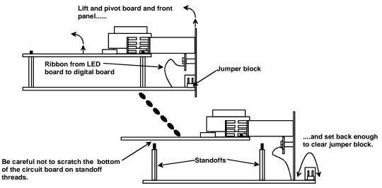
Set video board and front panel assembly back far enough to clear jumper block.
